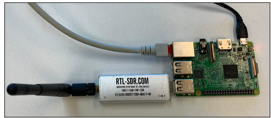
Fig. 2: The RU is comprised of a Raspberry Pi and an RTL-SDR
